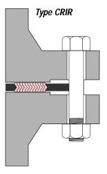
Solid metal outer and inner rings. For use at high pressures and
