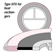
Spiral wound sealing element. Wound high density. Wide choice of materials for metal strip and filler material. For use in high-pressure pumps, high-pressure valves and gas applications. Low emission tested. graphite facing 0.5 mm. For use in manhole gaskets. Suitable for use with low bolt loads and uneven gasket surfaces. Double sealing effect. Combined inner and outer rings. The inner ring could have pass bars or could carry either a metal clad or soft gasket with pass bars.
