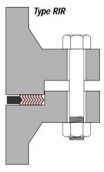
Solid metal inner ring. Use with high pressures and temperatures. Male to female flanges.
