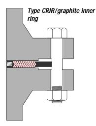
Solid metal inner ring with graphite facing. For use at high pressures and temperatures. Suitable for raised face or flat face flanges. Suitable for corrosive media. Graphite inner ring acts as an additional gasket.
