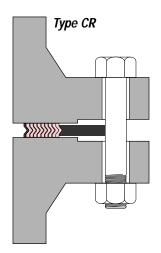
Wide choice of materials for metal strip and filler. Suitable for high pressures and temperatures. Recommended for flanges with tongue and groove. Solid metal outer ring used as a centerring device and compression stop. Used on raised face and flat face flanges.
